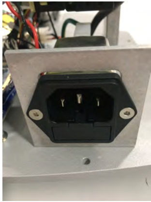
Figure 1: Fuse changing procedure
