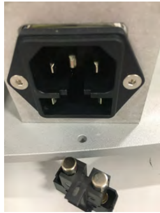
Figure 1: Fuse changing procedure
